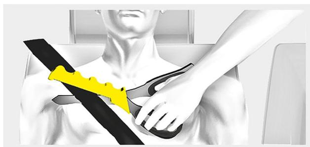
Used to cut seatbelts.
