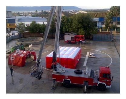
The rescue cushion is composed of two inflatable chambers, the first upper chamber acts as a large area of the first impact, the second lower chamber acts as a small area of the second impact.
